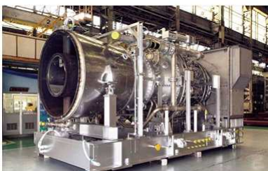
Mitsubishi Power 40-MW class ammonia gas turbine, 2021
