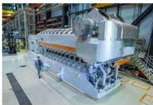
Wartsila 4 stroke engine fueled by NH 3 , 2020
